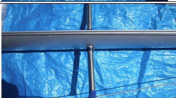
**Bad Idea:** This spreader is a straight through stainless tube, with two external sleeve each side riveted to hold it, both sides of the mast. It is a Flight mast, and it was the way we used to do the old Spunspar wing masts, no longer available. You can see the big gap 9mm left between the mast and the bottom sleeve, with a poorly fitted sleeve. Allowing the spreader to slide about in the mast hole, each tack the wire pressure will bring on the mast
