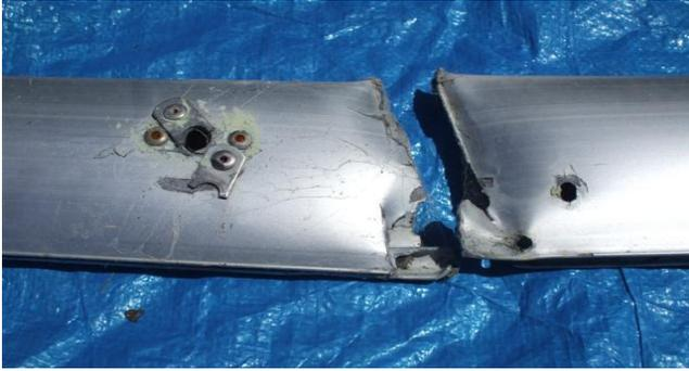
This mast was seven years old when it compressed at the gooseneck. The holes in the fittings show the reaction that has gone through three different owners use. Between the salt water, alloy and the loose stainless rivets and goose neck fitting, fractures started and the holes got bigger. Eventually under pressure of race conditions this Flight mast retired.
