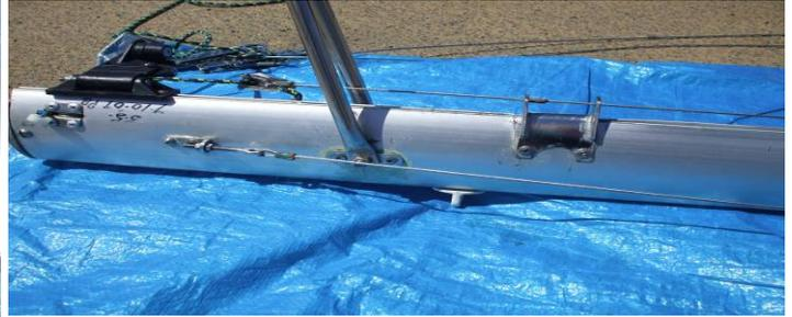
This Flight mast was installed in a Ns the same year as previous picture, but has lasted nine years, and over four owners. Having in November, had a sleeve pushed inside the mast from the bottom to just past the gooseneck and all the fittings refastened. Between the gooseneck bottom and rotator can be seen the area, the loose gooseneck fitting was wearing the mast. There are still small fractures in the mast where the rivets, are holding the gooseneck into the new insert internal alloy sleeve.
