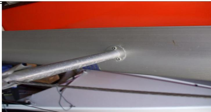
**Bad Idea:** This on a Aero ten Flight mast, which shows it required an extra alloy cover with two rivets each side of the mast for each spreader. The external spreader also requires a rivet to lock on to the internal tube through the mast. My guess would be the installation “stuffup” was due to having the original hole in the mast too big, to align the spreaders. So additional alloy is required to cover the big hole, and also stop spreader movement on the mast side.
